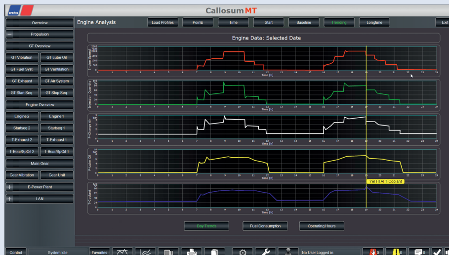
Figure 6: The trending function for relevant engine metrics helps to prevent damage.
