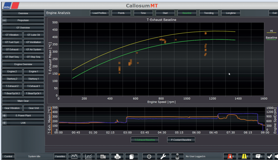
Figure 7: Baseline analysis helps to identify potential faults before they occur.
