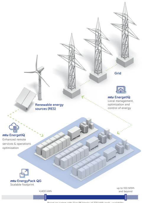
Based on system with 12 to 96 blocks of 370 kWh each - scalability up to 100 MWh and more beyond
