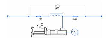
mtu Kinetic PowerPack protects the load
