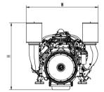
Dimensions (L  $\times$  W  $\times$  H): 1.817mm  $\times$  1.445mm  $\times$  1.349mm Weight (dry): 2.170kg All dimensions and weights are approximate.
