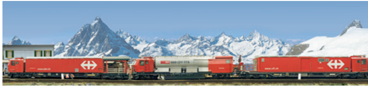
Fire fighting and rescue train
