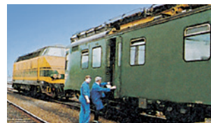
Overhead line inspection railcar
