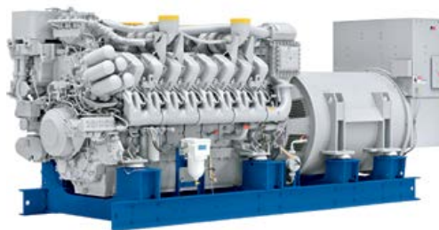
Three Type DS 2595 D5S emergency gensets are powered by three MTU Type 16V 4000 G63 diesel engines which produce 5,190 kVA of electric power. (Pictures: Robert Hack/MTU)
