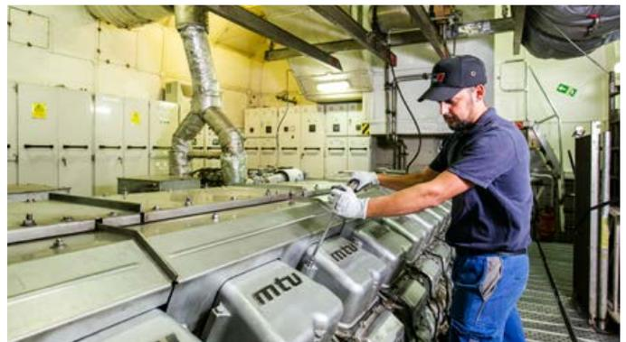
vessel. Engines from other MTU series can also undergo QL4 maintenance on the ship if the conditions are right for replacing the main bearings.
