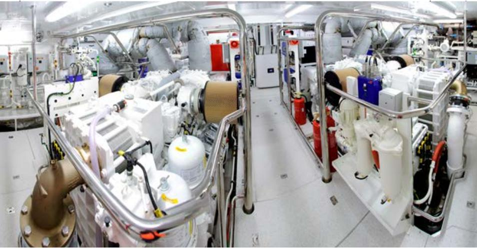
The power required for the propulsion of the new Sunseeker 155 is delivered by two MTU 12V 4000 M73L engines. Each engine boasts a rated power of 2,160 kilowatts at 2,050 rpm, enabling vessel speeds of up to 22 knots (41 km/h). (Photos: Rolls-Royce)
