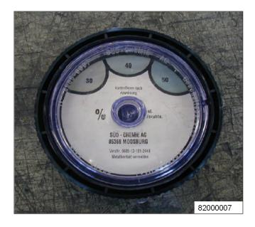
Note: The air humidity inside the packaging must be checked regularly every 3 to 4 months (→ Page 107). Measures to be carried out in case of changes to the relative air humidity are listed in the following table.
