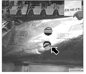
Screw the humidity indicator and vision panel into the laminated aluminum foil.
