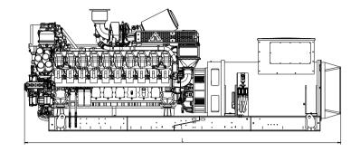
Drawing above for illustration purposes only, based on a standard open power 11 kV engine-generator set. Lengths may vary with other voltages. Do not use for installation design. See website for unit specific template drawings.
