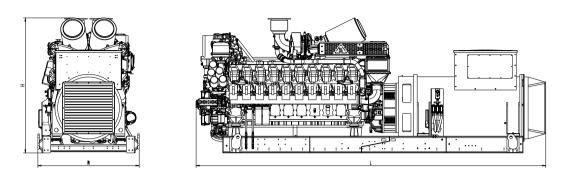
Drawing above for illustration purposes only, based on a standard open power 11 kV engine-generator set. Lengths may vary with other voltages. Do not use for installation design. See website for unit specific template drawings.
