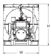
Drawing above for illustration purposes only, based on standard open power 480 volt generator set. Lengths may vary with other voltages. Do not use for installation design. See website for unit specific template drawings.
