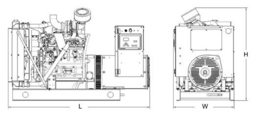
Drawing above for illustration purposes only, based on standard open power 400 volt generator set. Lengths may vary with other voltages. Do not use for installation design. See website for unit specific template drawings.
