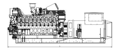
Drawing above for illustration purposes only, based an standard open power 11 kV engine-generator set. Lengths may vary with other voltages. Do not use for installation design. See website for unit specific template drawings.
