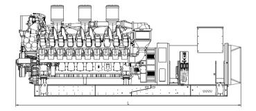
Drawing above for illustration purposes only, based on a standard open power 400 Volt engine-generator set. Lengths may vary with other voltages. Do not use for installation design. See website for unit specific template drawings.
