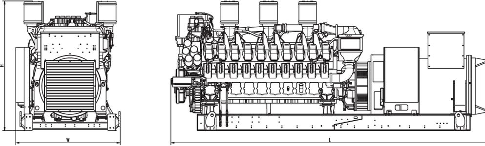
Drawing above for illustration purposes only, based on a standard open power 400 Volt engine-generator set. Lengths may vary with other voltages. Do not use for installation design. See website for unit specific template drawings.
