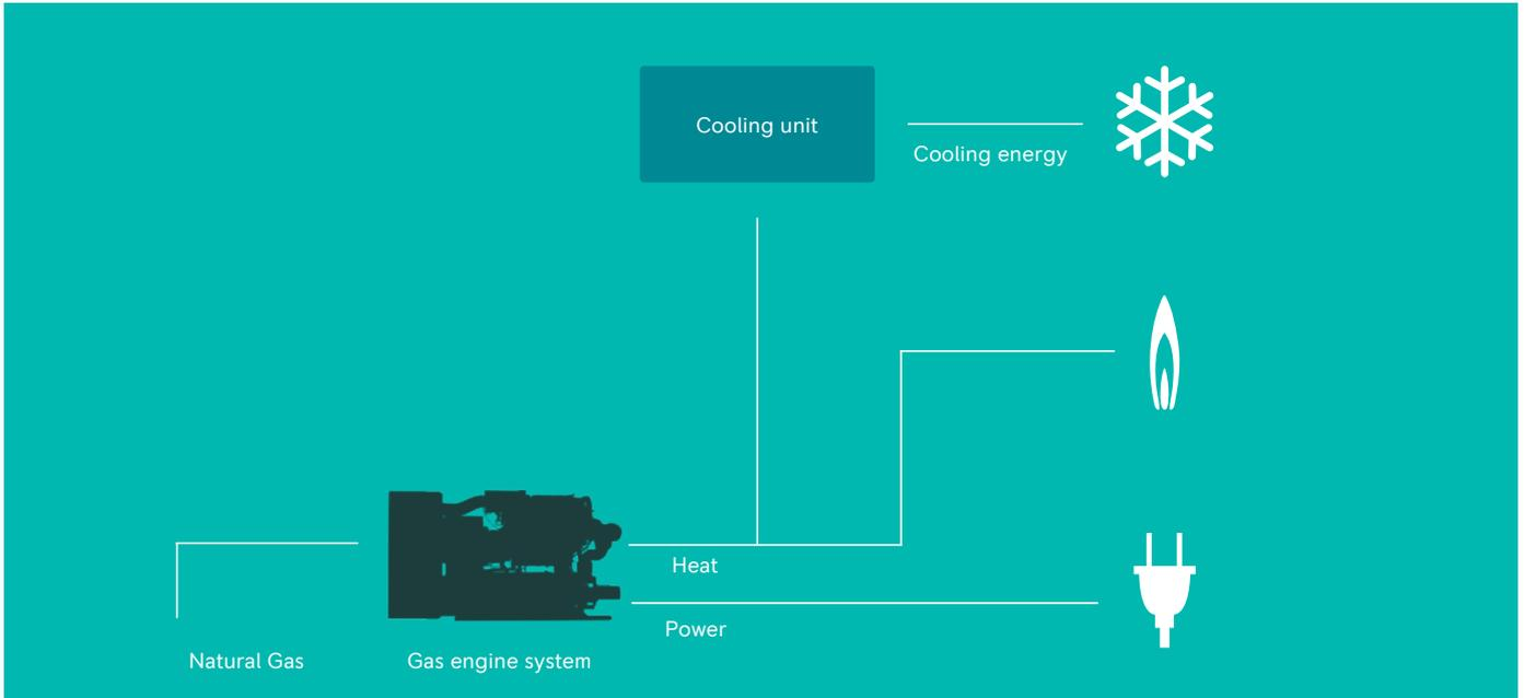
Using a cooling unit such as an absorption or adsorption chiller, CHP systems can also create cooling energy with their generated heat.
