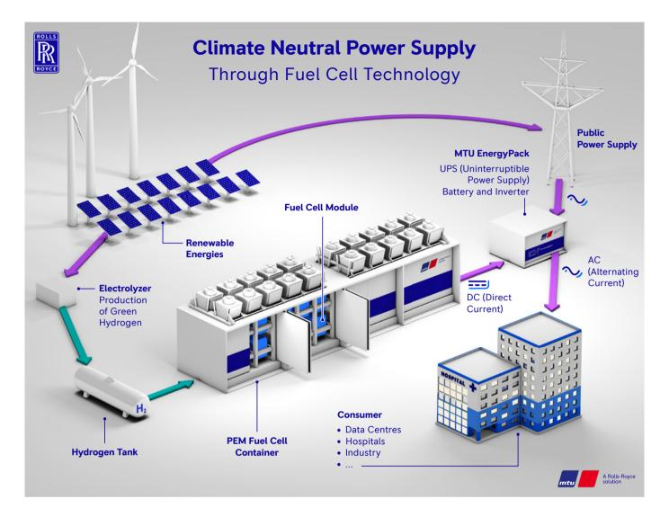
Rolls-Royce Power Systems is aiming to offer an integrated, fullyfeatured emergency power solution. This will include the fuel cell system, a UPS system, batteries and the hydrogen infrastructure. The solution will be black-start-capable, i.e. able to resume generation without intervention, and deliver more than two MW of power.
