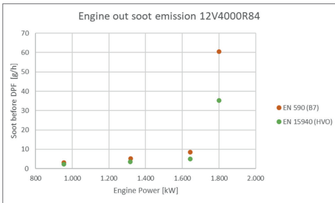
Figure 7: Soot emissions upstream of the DPF on a 12V4000R84 unit
